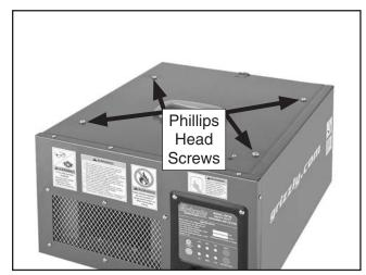
Figure 8. Remove these Phillips head screws.
